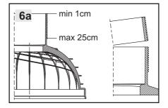
A taper should be installed similarly to other manhole components (rings Ø1000) A cylindrical section of the taper (from the minimum of 1 to the maximum of 25 cm) may be cut to achieve the required manhole height.
